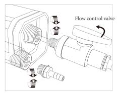
This flow is designed for the measurement of residual chlorine by potentiostatic method and can also be combined with other sensors. The design principle allows the sample to pass through the electrode position at a constant speed through the check valve to adjust the flow rate
