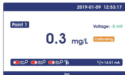
**Point 1 calibration:** After entering the calibration mode, the instrument displays as shown in the figure above. The main value of the instrument displays the known standard liquid value of point 1.Place the electrode into the standard solution of the corresponding value, and the corresponding voltage mV value and calibration state will be displayed on the left side of the screen.
